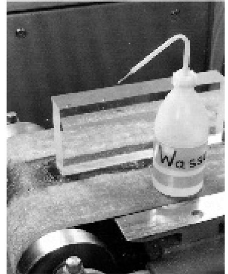
Fig. 38: Wet sanding on a belt sanding machine
