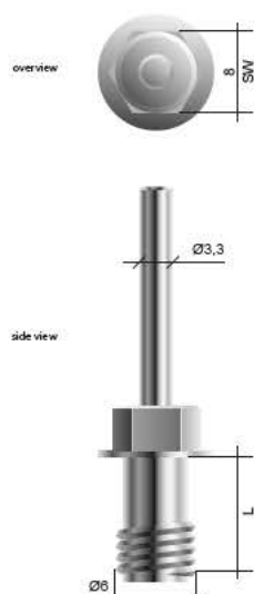
Fig. Clinch bolt – Construction and dimensions (mm).
