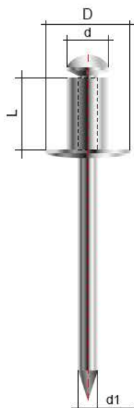
Fig. Blind rivet – construction and dimensions.
