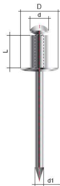
Fig. Blind rivet - construction and dimensions.
