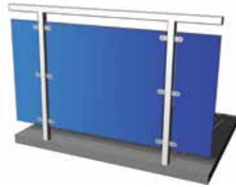
Fig. Fixing to the posts using fasteners or clamping chucks.
