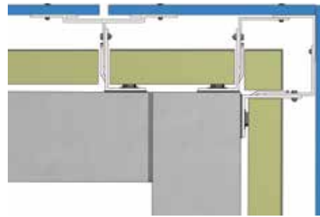
Fig. Ventiladed facades - horizontal cross-section.
