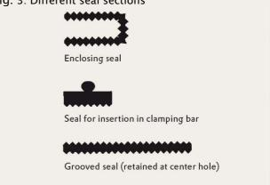
The sealing sections used determine the watertightness of glazing with PLEXIGLAS®. Particularly important is the material they are made of. PLEXIGLAS® is sensitive to certain sealants, which should therefore always be tested for compatibility.
