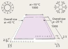
Because of the possible change in length, the clamping depth of the glazing should be between 15 and 20 mm. In addition, there is to be a clearance "a" for expansion and compensation for building tolerance. The value "a" depends on the sheet size and corresponds to one half of the general expansion allowance calculated as above (Fig. 2).
