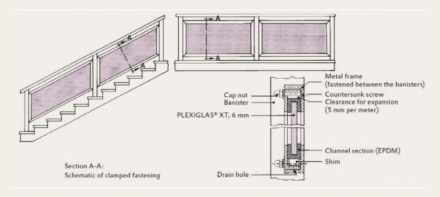
Fig. 9: Clamping on two sides
