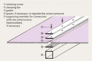
As a general principle, linear fastening is to be preferred since the load conditions are more favorable in this case and thinner sheets can be used as a result. The allowance to be made for expansion is again 5 mm/m for PLEXIGLAS® (PLEXIGLAS® Resist: 6 mm/m).
