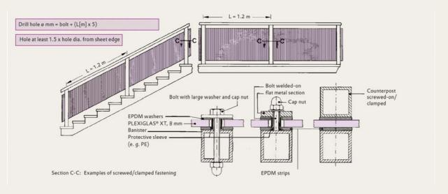
Fig. 11: Pointwise fastening
