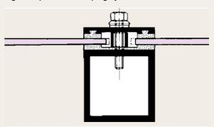
Fig. 6: Too high clamping pressure
