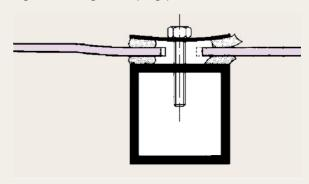
Fig. 7: Spacer sleeve (also for edge protection)
